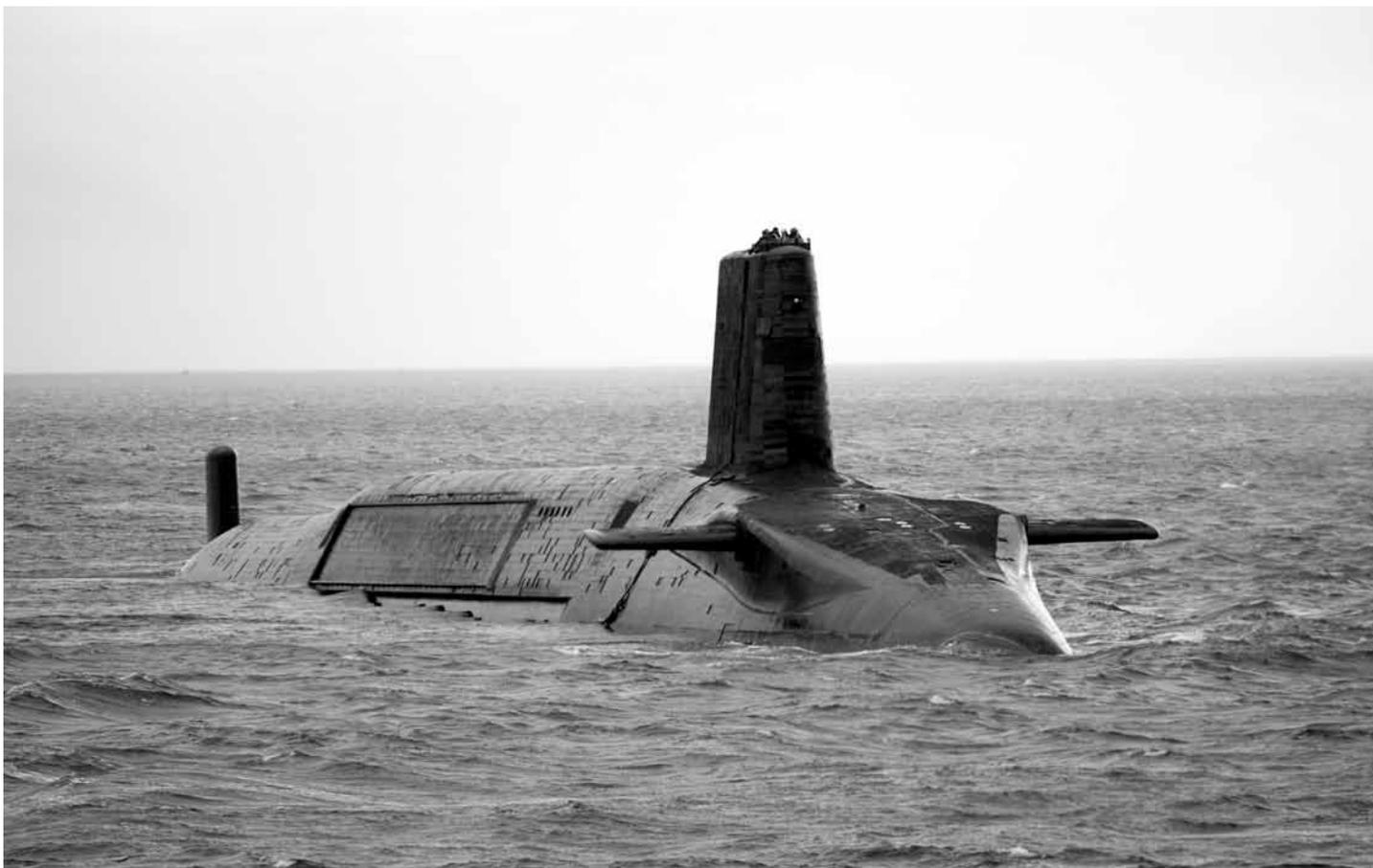
**The HMS Vigilant, shown off the coast of Scotland in 2012, is one of four UK Vanguard-class SSBNs, whose nuclear propulsion reactors run on weapons-grade uranium. The Royal Navy is planning to replace these submarines with the Successor-class, powered by a new reactor, starting around 2028. U.S. Ohio-class SSBNs also use weapons-grade uranium fuel and are scheduled to be replaced with the SSBN(X), starting in 2029.**
